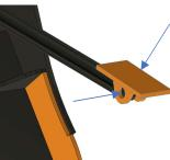
8. Lift the boom to a suitable height and securely clamp the mount centrally on the arm. The ideal distance from the quick hitch pin is when the cylinder is fully retracted but not parallel to the arm.
