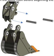
2. Lower the quick hitch to the ground and remove the front pin. If a hydraulic quick hitch is installed, please ensure, throughout the installation process, that its hydraulic hoses are not over-stretched or pinched at any point.
