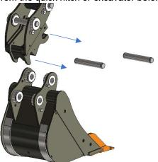
2. Lower the quick hitch to the ground and remove the front pin of the quick hitch. If a hydraulic quick hitch is installed, please ensure, throughout the installation process, that its hydraulic hoses are not over-stretched or pinched at any point.
