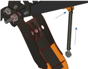
7. Manipulate the top of the cylinder into the thumb mount and pin in place with the supplied pin and retention hardware.
